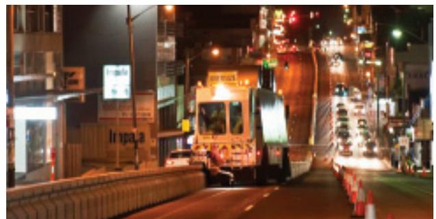
Figure 17. Moveable lane barrier vehicle in operation. Courtesy of Roads and Maritime Services, New South Wales
